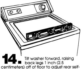
centimeters) off of floor to adjust rear selfleveling legs. Gently lower washer to floor. Check levelness of the washer by placing a carpenter's level on top of the washer, first side to side; then front to back.
